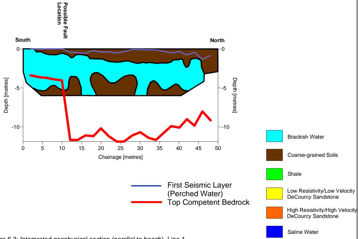
Figure 6.3: Interpreted geophysical section (parallel to beach), Line 1, Roes Island, North Pender Island
