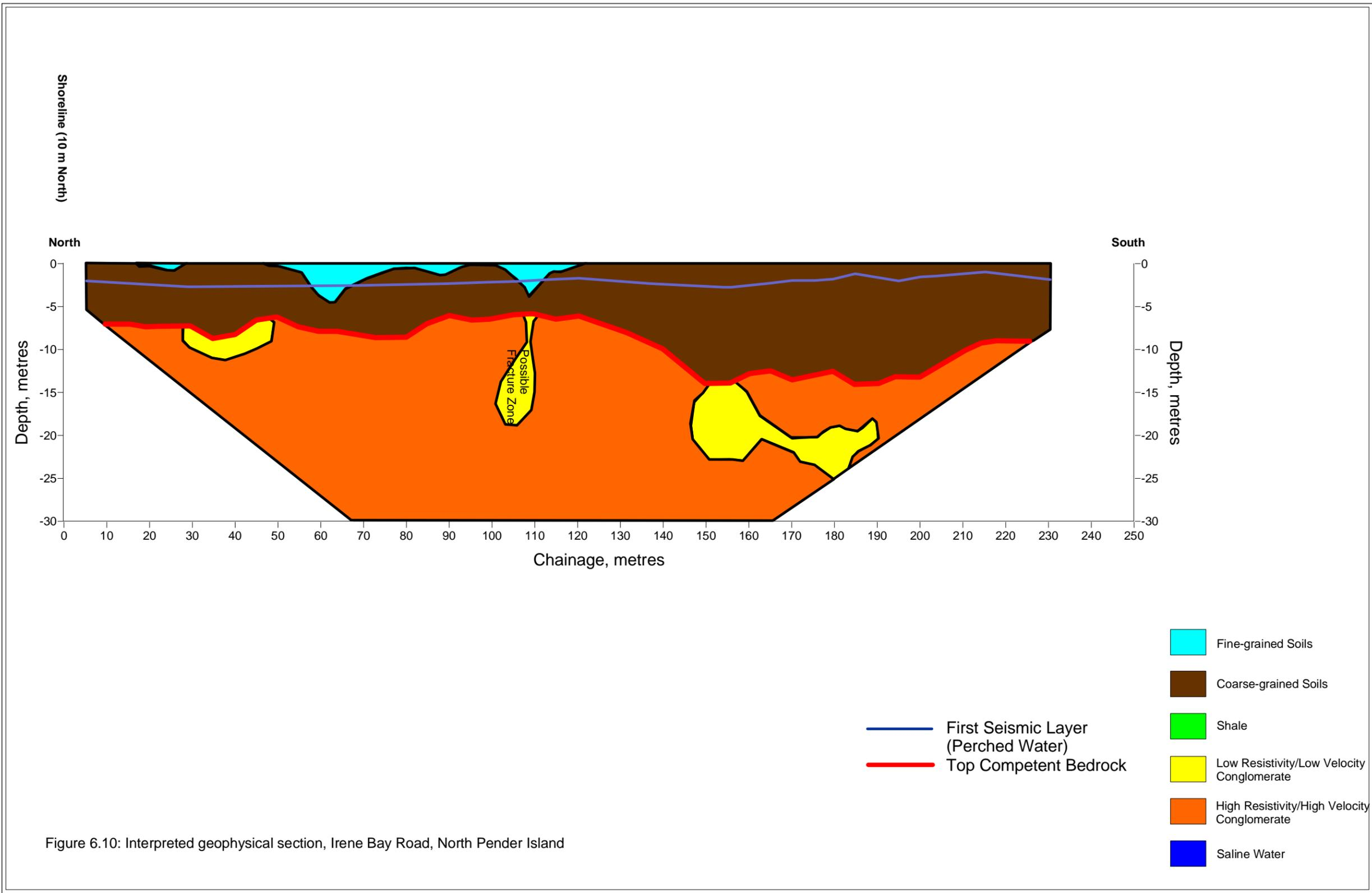
Figure 6.10: Interpreted geophysical section, Irene Bay Road, North Pender Island
