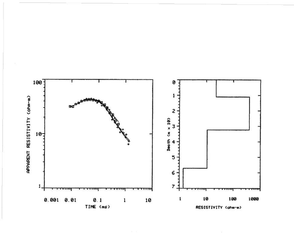
Figure 6.7: Time domain electromagnetic sounding at Roes Islet, North Pender Island. The apparent resistivity curve on the left illustrates the field data along with the model curve that fits the data. The model used is shown on the right.
