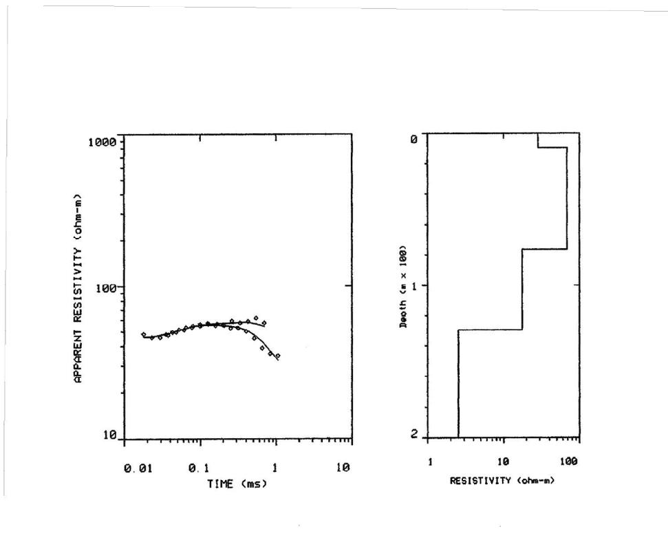
Figure 6.36: Time domain electromagnetic sounding beside Spalding Road, South Pender Island. The apparent resistivity curve on the left illustrates the field data along with the model curve that fits the data. The model used is shown on the right.
