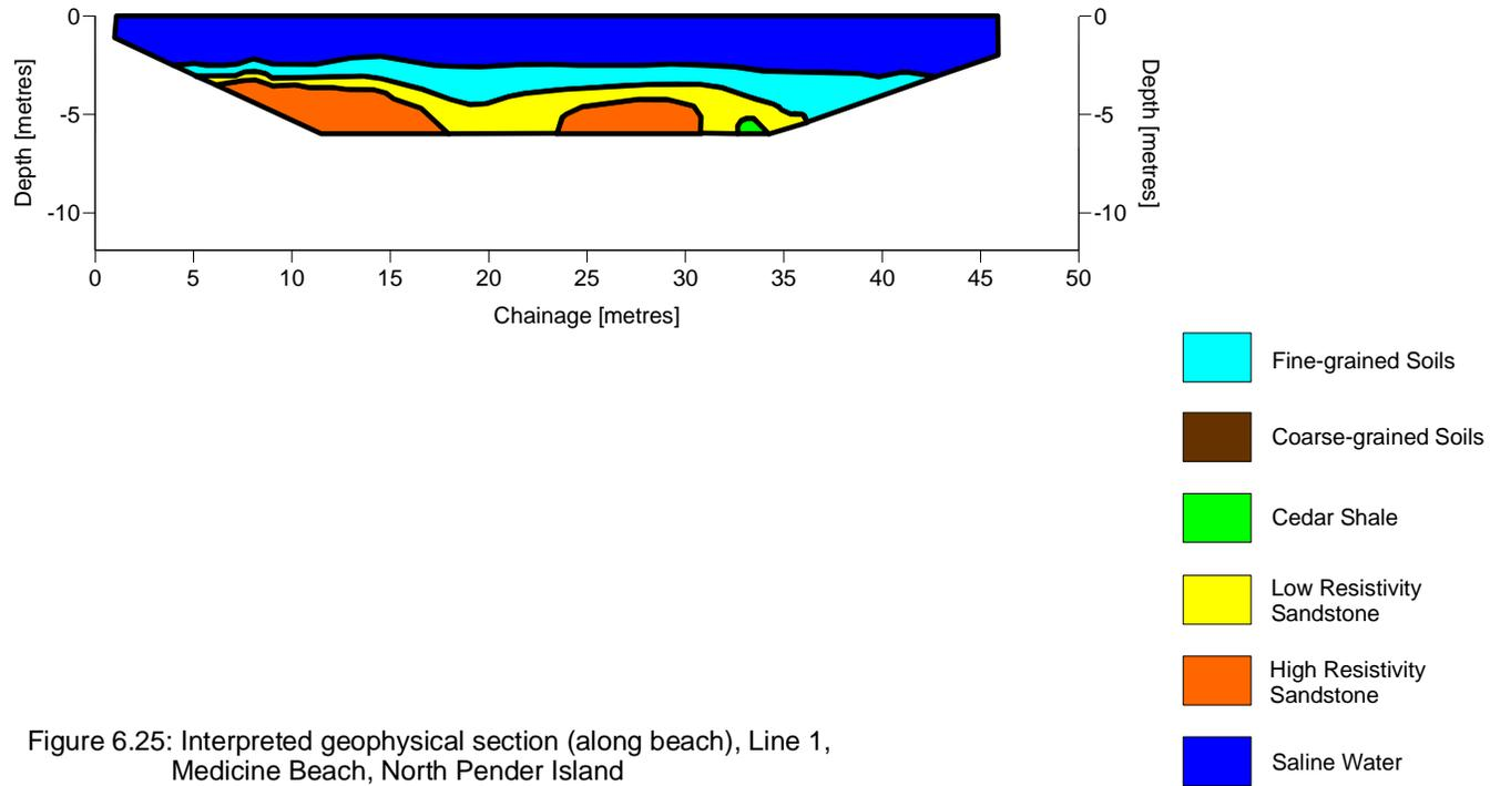
Figure 6.25: Interpreted geophysical section (along beach), Line 1, Medicine Beach, North Pender Island
