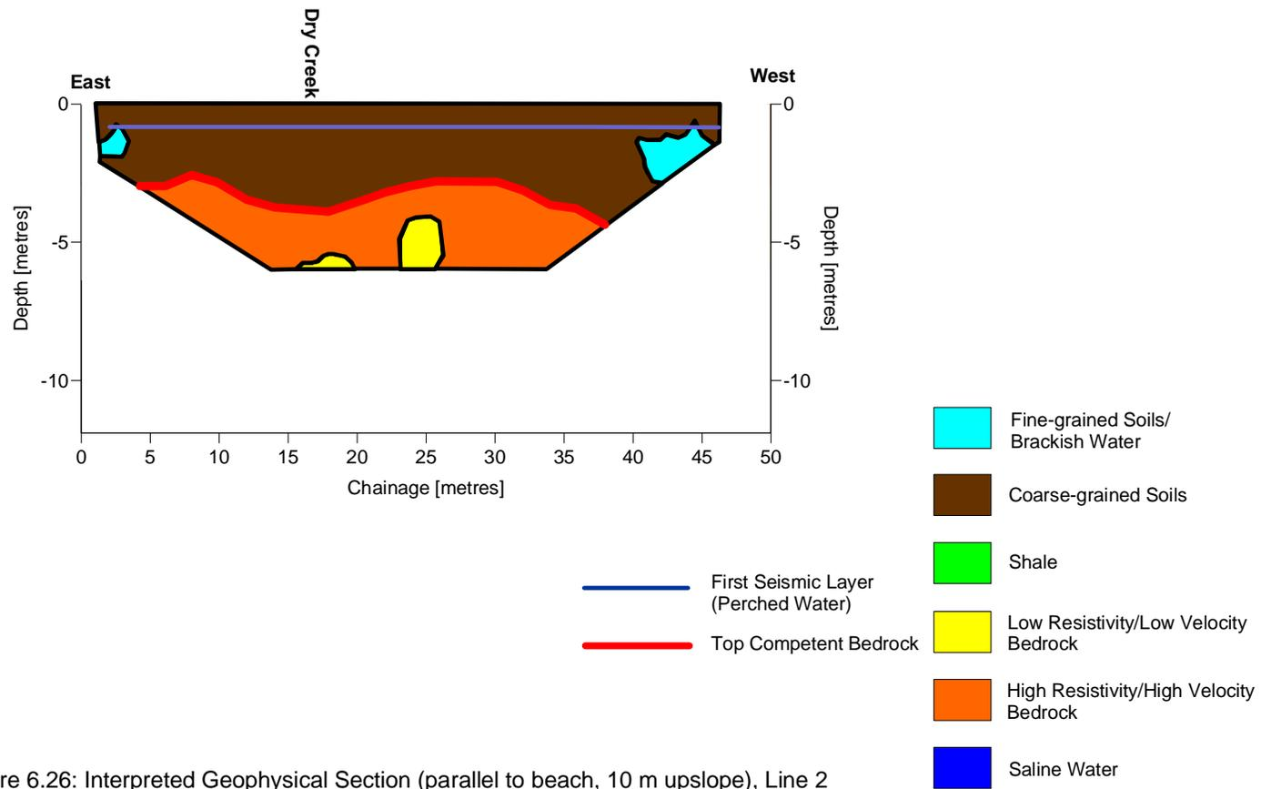
Figure 6.26: Interpreted Geophysical Section (parallel to beach, 10 m upslope), Line 2 Medicine Beach, North Pender Island
