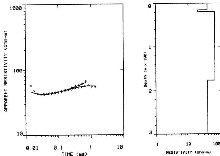
Figure 6.18: Time domain electromagnetic sounding beside Community Hall, North Pender Island. The apparent resistivity curve on the left illustrates the field data along with the model curve that fits the data. The model used is shown on the right.
