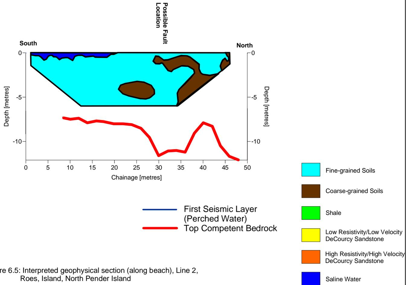
Figure 6.5: Interpreted geophysical section (along beach), Line 2, Roes Island, North Pender Island
