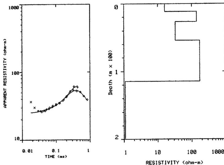
Figure 6.16: Time domain electromagnetic sounding beside Hoosen Road, North Pender Island. The apparent resistivity curve on the left illustrates the field data along with the model curve that fits the data. The model used is shown on the right.
