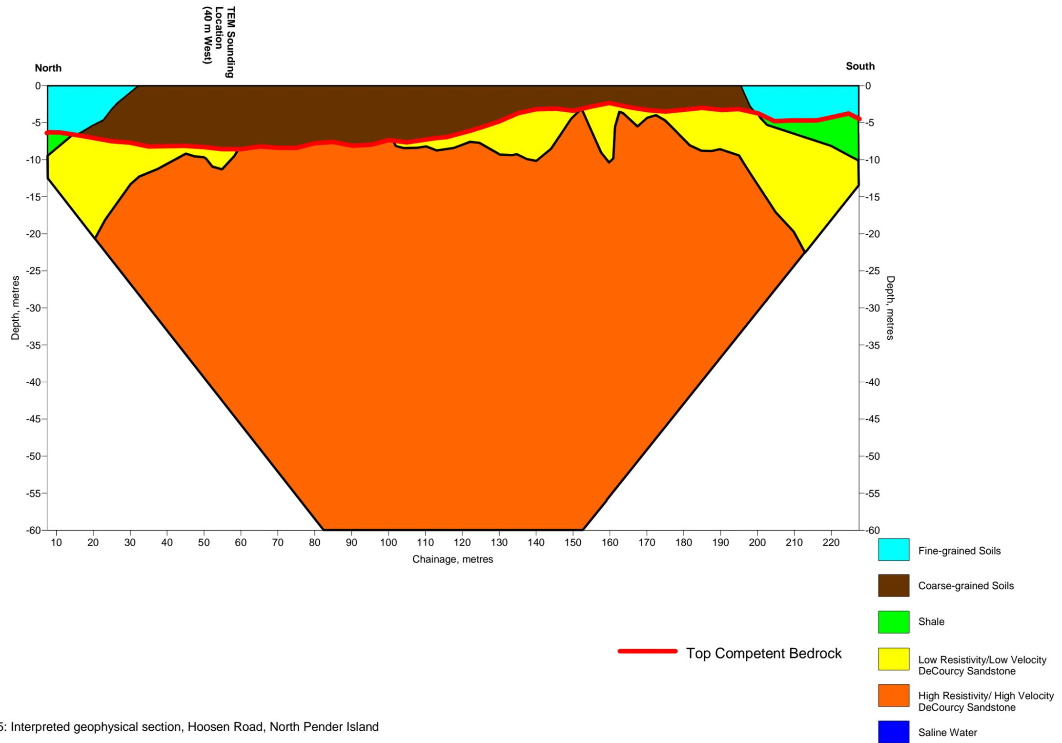
Figure 6.15: Interpreted geophysical section, Hoosen Road, North Pender Island
