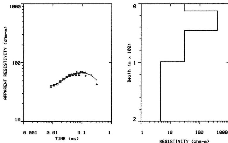
Figure 6.8: Time domain electromagnetic sounding at Roes Islet, North Pender Island. The apparent resistivity curve on the left illustrates the field data along with the model curve that fits the data. The model used is shown on the right. This sounding is located 10 metres upslope from the sounding shown in Figure 6.7.
