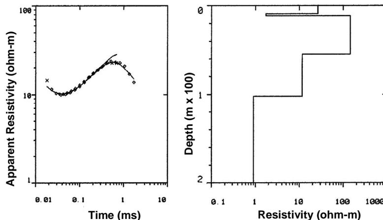
Figure 6.29: Time domain electromagnetic sounding beside Medicine Beach, North Pender Island. The apparent resistivity curve on the left illustrates the field data along with the model curve that fits the data. The model used is shown on the right.
