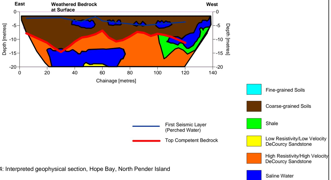
Figure 6.14: Interpreted geophysical section, Hope Bay, North Pender Island
