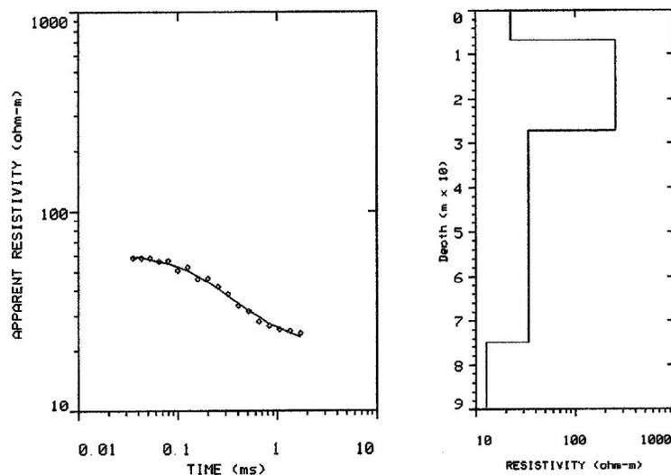
Figure 6.13: Time domain electromagnetic sounding along Corbett Road, North Pender Island. The apparent resistivity curve on the left illustrates the field data along with the model curve that fits the data. The model used is shown on the right.
