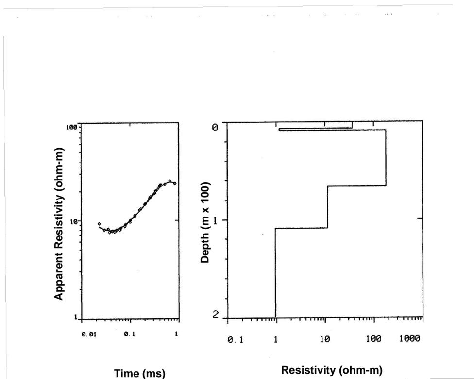
Figure 6.30: Time domain electromagnetic sounding beside Medicine Beach, North Pender Island. The apparent resistivity curve on the left illustrates the field data along with the model curve that fits the data. The model used is shown on the right.
