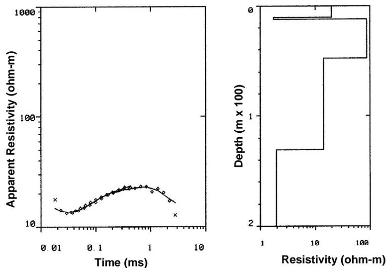
Figure 6.31: Time domain electromagnetic sounding beside Medicine Beach, North Pender Island. The apparent resistivity curve on the left illustrates the field data along with the model curve that fits the data. The model used is shown on the right.
