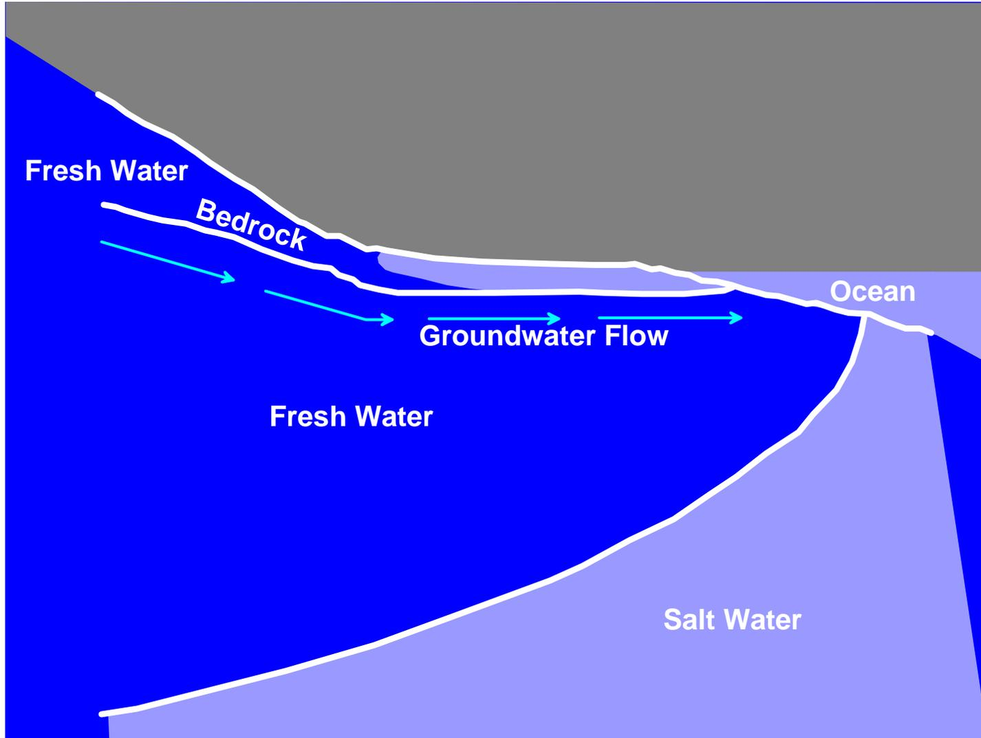
Figure 6.27: Conceptual groundwater flow model, Medicine Beach, North Pender Island
