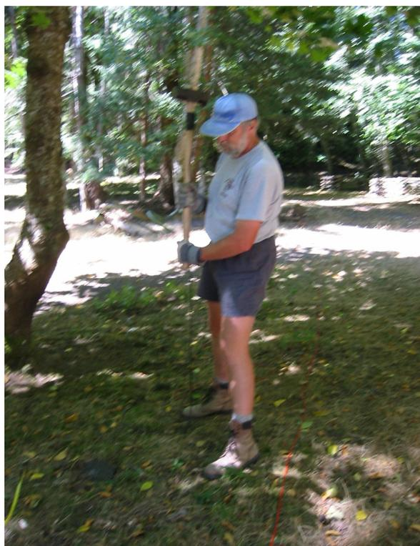
Figure 2.7: Sledge-hammer as seismic energy source
