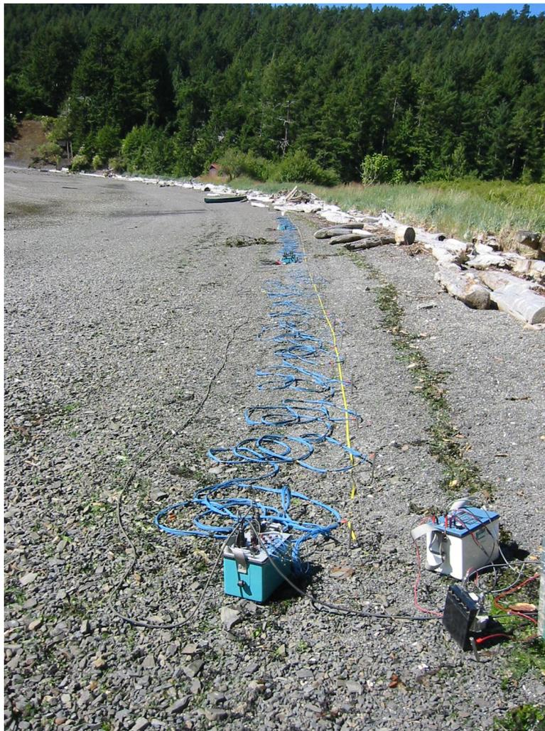
Figure 2.10: Electrical Imaging array, Medicine Beach, North Pender Island
