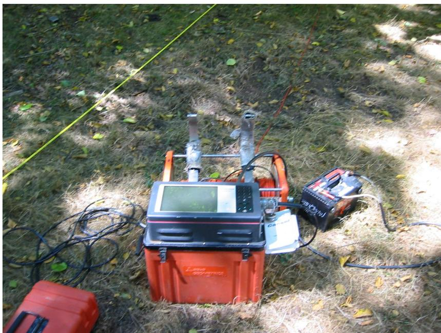
Figure 2.6: Seismograph and power supply
